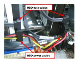
11. Disconnect the HDD data cables from the main board.
